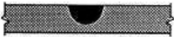
ACHF DEEP PENETRATION-WIDE WELD
